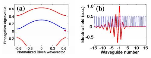
Fig. 5. (a) Band structure of the composite array showing the first order bands of the right-side array (red, top) and of the left-side array (blue, middle), and part of the second order band (red, bottom) of the right-side array. (b) Electric field distribution associated with the interface mode.
