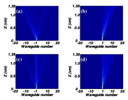
Fig. 3. Simulated discrete diffraction intensity patterns when the distance between arrays is decreased. (a), (b) d=3 µm; (c), (d) d=2 µm. Boundary channel of the left-side (a), (c) and right-side (b), (d) arrays was excited.
