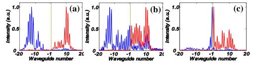
Fig. 4. Intensity patterns observed at the output facet of AlGaAs samples for different separations between two arrays for (a)  $d = 4 \mu m$ , (b)  $d = 3 \mu m$ , and (c)  $d = 2 \mu m$ . Intensity distributions when the first channel of the left (blue curves) and of the right (red curves) array is excited are shown. The position of the interface is shown by a dotted line.
