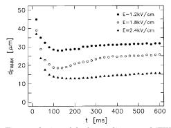
Fig. 4. Time evolution of the beam diameter d (FWHM) in the presence of different externally applied electric fields E. The input power of the He–Ne laser light is 55  $\mu$ W.
