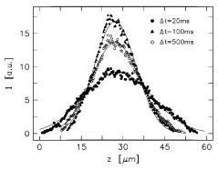
Fig. 5. Intensity profiles I(z) at the exit face of the waveguide measured for different time delays  $\Delta t$  after the He–Ne laser beam is switched on. The profiles are for the measurement shown in Fig. 4 and E = 1.8 kV/cm.
