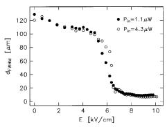
Fig. 2. Beam diameter *d* (FWHM) at the exit face of the waveguide as a function of the electric field *E* for two different input powers  $P_{\rm in}$  of He–Ne laser light. The background illumination with green light ( $\lambda = 514.5$  nm) is ~30 mW/cm<sup>2</sup>. All diameters are measured in the steady state.
