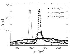
Fig. 3. Intensity profiles I(z) at the exit face of the waveguide measured for different externally applied electric fields E. The profiles are for the measurement shown in Fig. 2 and an input power  $P_{\rm in} = 4.3 \ \mu W$ . For comparison, the solid curve shows the input beam profile (shifted for better viewing).
