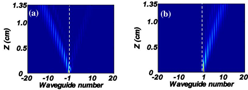
Fig. 2. BPM simulations for  $d = 4 \mu\text{m}$  when a single boundary channel of the left (a) and right (b) arrays was excited, respectively. The position of the interface is shown by a dashed line;  $Z$  is the propagation distance.
