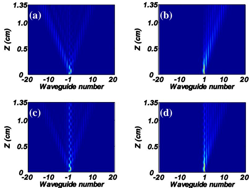
Fig. 3. Simulated discrete diffraction intensity patterns when the distance between arrays is decreased. (a), (b)  $d = 3 \mu\text{m}$ ; (c), (d)  $d = 2 \mu\text{m}$ . Boundary channel of the left-side (a), (c) and right-side (b), (d) arrays was excited.
