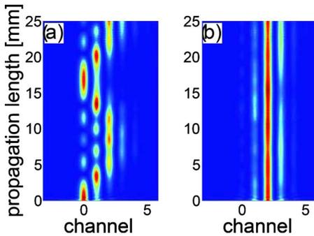
Fig. 4. (Color online) Saturable defocusing WA with input profile and lattice parameters from Fig. 3, but  $\Delta n_{nl} = 6.21 \times 10^{-4}$  and  $r = 6$ . Input beam is launched into (a) first and (b) third channels.
