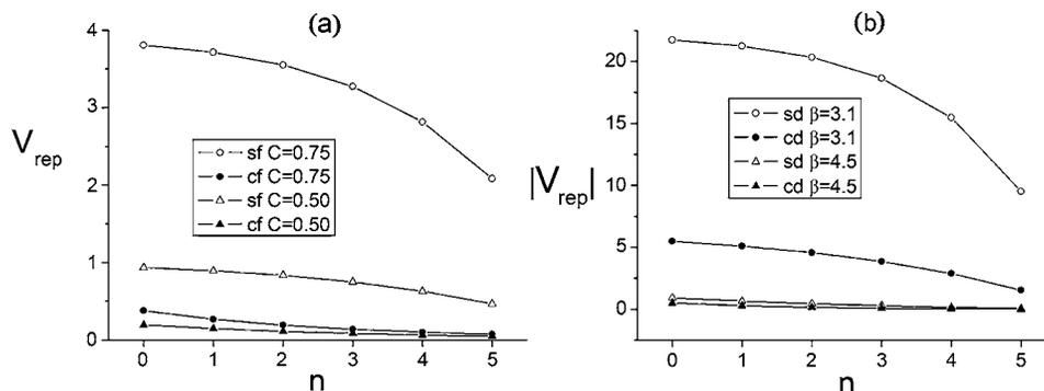
Fig. 2. Dependence of the effective repulsive potential on the distance from the boundary. (a) Self-focusing case:  $|\beta|=3.1$ ,  $|F_0|^2=0.24$ , and different values of  $C$ . (b) Self-defocusing case:  $C=0.5$ ,  $|F_0|^2=0.172$ , and different values of  $\beta$ .
