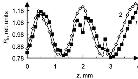
Fig. 3. Spatial dependences of the normalized optical power transmitted through the LiNbO<sub>3</sub>: Fe: Cu sample before (curve 1) and after exposure to the probing beam (curve 2).
