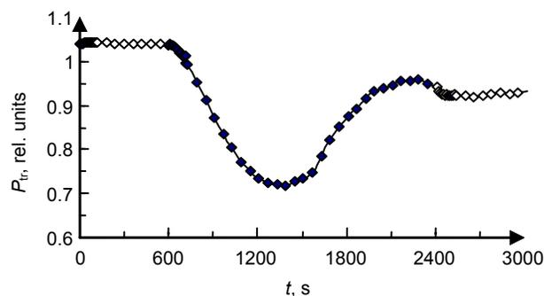
Fig. 6. Time dependence of normalized transmitted optical power for the LiNbO<sub>3</sub>: Fe: Cu sample with Fe and Cu diffusion depths of 50 μm under continuous background illumination. Illumination was switched on at  $t = 600$  s and switched off at  $t = 2400$  s.
