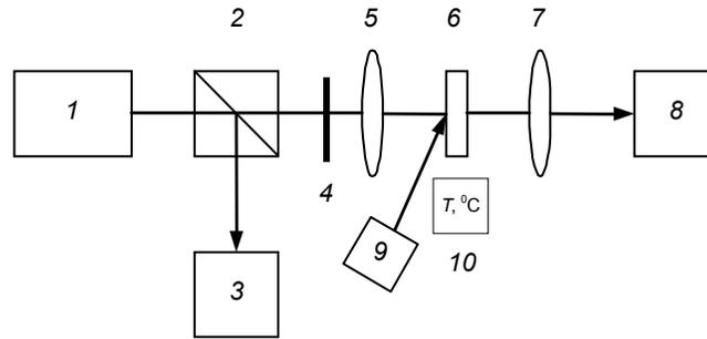
Fig. 1. Scheme of the experiment on the study of the optical transmission of samples comprising He-Ne laser 1, beam-splitting cube 2, photo diode 3, optical filter 4, focusing lens 5, examined sample 6, imaging lens 7, photodiode 8, light-emitting diode 9, and thermometer 10.
