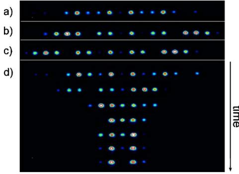
FIG. 2. (Color online) Discrete diffraction (a)–(c) and nonlinear interaction (d) of two copropagating in-phase beams. The photographs show the corresponding images on the output facet of the NWA when (a) both beams are present; (b),(c) one beam is blocked, and (d) time evolution of two-beam interaction for an input power of  $P \approx 7 \mu\text{W}$ .
