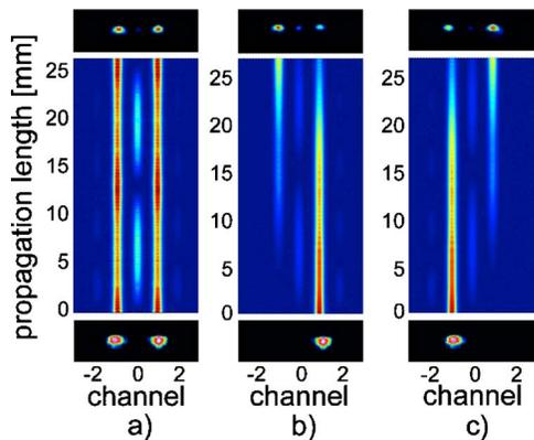
FIG. 4. (Color online) Read-out of light-induced structures. Upper/lower parts: images from the input facet (top) and the corresponding images from the output facet (bottom). Middle parts: numerical simulation of build-up (a) and single beam propagation (b),(c) in the induced structure. (a) Initial two-beam interaction; (b) and (c) read-out of the induced structure with a probe beam coupled in the left or right input channel, respectively.
