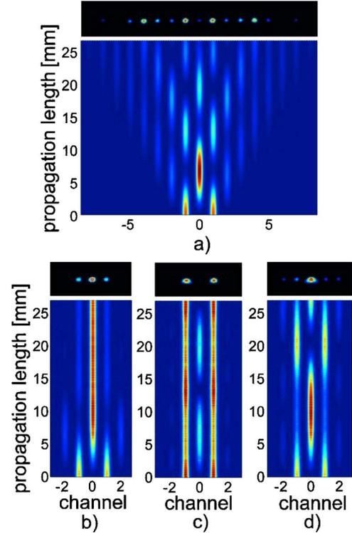
FIG. 3. (Color online) Comparison of in-phase interaction for different input powers and saturable nonlinearity. (a) Discrete diffraction. (b) Soliton fusion:  $P \approx 0.5 \mu\text{W}$ ,  $r=0.43$ . (c) Solitonlike propagation:  $P \approx 7 \mu\text{W}$ ,  $r=4.62$ . (d) A wide structure  $P \approx 25 \mu\text{W}$ ,  $r=30$ .
