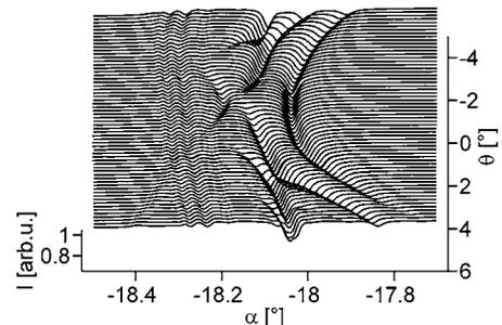
Fig. 3. Full spectrum of reflected light intensity  $I$  as a function of incident angle  $\alpha$  and tilt angle  $\theta$ .
