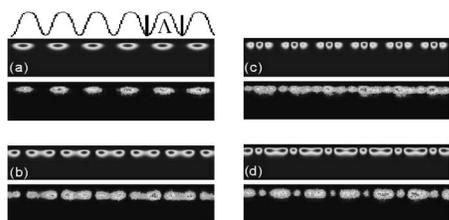
Fig. 5. Measured (lower part) and calculated (upper part) intensity distributions of extended FB modes at the output face for (a) band 1 at  $k_z = \pi/\Lambda$ , (b) band 2 at  $k_z = \pi/\Lambda$ , (c) band 3 at  $k_z = \pi/\Lambda$ , and (d) band 3 at  $k_z = 0$ .
