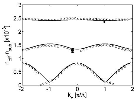
Fig. 4. Measured values (open symbols) and numerical modeling (solid curves) of the effective refractive indices  $n_{\text{eff}}$  of (linear) FB modes versus transverse wave vector  $k_z$ , relative to the substrate index  $n_{\text{sub}}$ . The solid square inside the gap is the measured effective index of an extended nonlinear mode.
