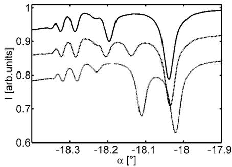
Fig. 2. Measured output light intensity  $I$  versus incident angle  $\alpha$  for three different values of angle  $\theta$  corresponding to  $k_z=0$  (solid curve),  $k_z=\pi/(2\Lambda)$  (dashed curve), and  $k_z=\pi/\Lambda$  (dotted curve).
