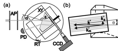
Fig. 1. (a) Prism coupling method: AP, apertures; XY, *xy*-stage; RT, rotary stage; PD, photodiode; CCD, CCD camera. (b) Adjustment of  $k_z$  by tilting the sample by an angle  $\theta$ .
