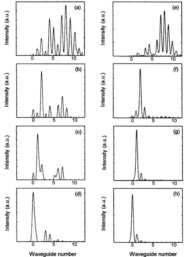
Fig. 3. Output patterns for single-channel excitation and four different input powers. Left column: experimental results for (a) discrete diffraction, (b)  $P=32.5 \mu\text{W}$ , (c)  $P=270 \mu\text{W}$ , and (d)  $P=450 \mu\text{W}$ . Right column: simulation results for (e) discrete diffraction, (f)  $P=32 \mu\text{W}$ , (g)  $P=275 \mu\text{W}$ , and (h)  $P=450 \mu\text{W}$ .
