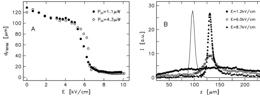
**Fig. 3.** Spatial soliton formation in a planar SBN waveguide. (A) Beam diameter  $d$  (FWHM) at the output face of the waveguide as a function of the electric field  $E$  and for two different input powers  $P_{\text{in}}$  of the HeNe laser. (B) Intensity profiles  $I(z)$  on the output face measured for different external electric fields  $E$  and for an input power of  $P_{\text{in}} = 4.3 \mu\text{W}$ . The solid line shows the input beam profile (shifted for better viewing)
