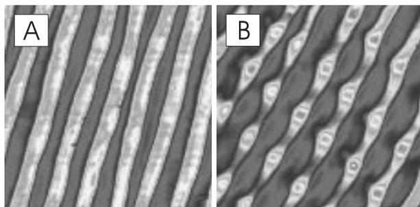
**Fig. 5.** Intensity at the output plane of the crystal. The correlation distance is  $l_c=13\ \mu\text{m}$  and the displayed area is  $0.5\times 0.5\ \text{mm}^2$ . Plot (A) shows the case above threshold where 1D filaments occur. For much higher nonlinearity the filaments become unstable and form a 2D pattern (B)
