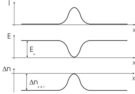
**Fig. 2.** Formation of a bright photorefractive soliton. In the region illuminated by a narrow beam the external electric field is screened, leading to a local positive refractive-index change via the electrooptic effect
