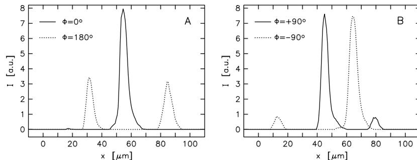
**Fig. 4.** Intensity distribution  $I(x)$  on the endface of a planar SBN waveguide for different relative phases  $\Phi$  of the two solitons. The two solitons intersect at an angle  $2\theta \approx 0.7^\circ$  and their separation on the endface without interaction is  $35 \mu\text{m}$ . (A)  $\Phi=0^\circ$  (solid line) and  $\Phi=180^\circ$  (dotted line). (B)  $\Phi=+90^\circ$  (solid line) and  $\Phi=-90^\circ$  (dotted line), both cases show energy exchange
