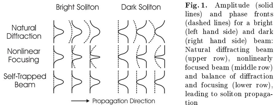
**Fig. 1.** Amplitude (solid lines) and phase fronts (dashed lines) for a bright (left hand side) and dark (right hand side) beam: Natural diffracting beam (upper row), nonlinearly focused beam (middle row) and balance of diffraction and focusing (lower row), leading to soliton propagation
