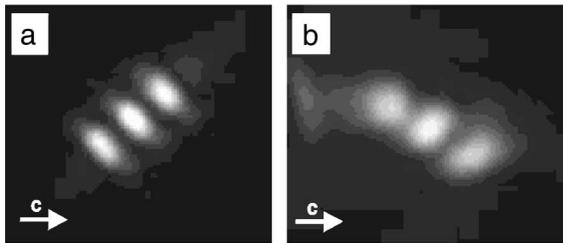
Fig. 3. Image of the three spots aligned at  $45^\circ$  with respect to the  $c$  axis: a, image beam on the input face; b, image beam on the output face with  $E = 7.2$  kV/cm and the soliton beam on. The  $c$  axes are marked by arrows. Picture size is  $50 \mu\text{m} \times 50 \mu\text{m}$ .
