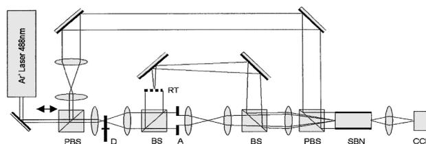
Fig. 1. Experimental setup: PBS's, polarizing beam splitters; D, rotating diffuser; BS's, beam splitters; RT, resolution target; A, aperture; SBN, nonlinear crystal; CCD, CCD camera.
