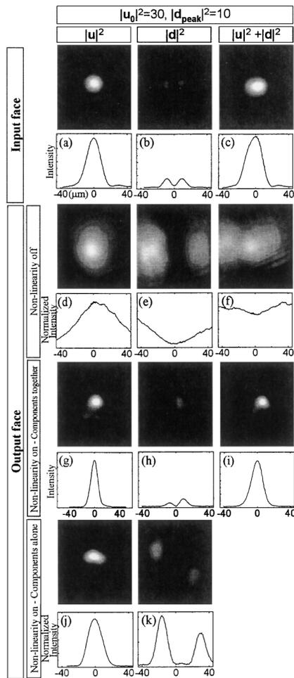
Fig. 2. Same as in Fig. 1 but with  $|u_0|^2 = 30$  and  $|d_{\text{peak}}|^2 = 10$ . This single-hump soliton forms for an applied field of 4060 V/cm.
