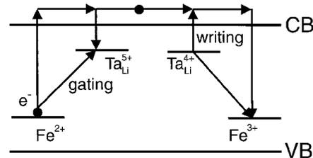
Fig. 2. Two-center charge-transport model in  $\text{LiTaO}_3:\text{Fe}$ . Deep center,  $\text{Fe}^{2+/3+}$ ; shallow center,  $\text{Ta}_{\text{Li}}^{4+/5+}$ ; VB, valence band; CB, conduction band.
