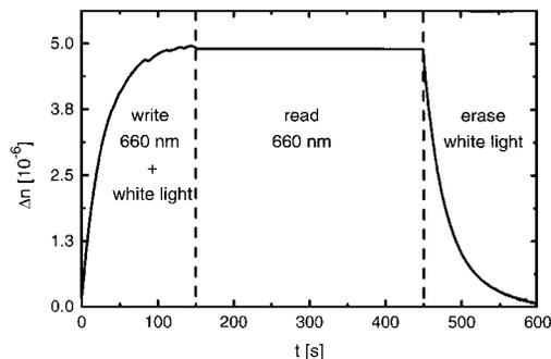
Fig. 1. Refractive-index change for a typical write-read-erase cycle. The hologram is recorded with a 660-nm diode laser ( $I_{\text{writing}} = 0.65$   $\text{W}/\text{cm}^2$ ) and white light from a Xe lamp for gating. Nondestructive readout is performed with one of the writing beams, and hologram erasure is possible with the gating light.
