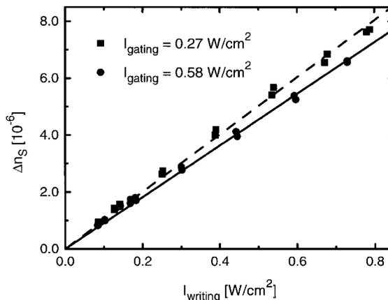
Fig. 3. Saturation values  $\Delta n_S$  of refractive-index changes as a function of the writing intensity  $I_{\text{writing}}$  for two different gating intensities. The lines are linear fits to the measured values.
