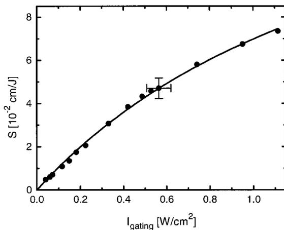
Fig. 5. Dependence of photorefractive sensitivity  $S$  on the gating intensity at 488 nm. The curve is a fit according to  $S = aI_{\text{gating}}/(b + I_{\text{gating}})$ .
