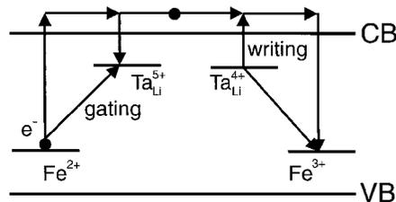
Fig. 2. Two-center charge-transport model in  $\text{LiTaO}_3:\text{Fe}$ . Deep center,  $\text{Fe}^{2+/3+}$ ; shallow center,  $\text{Ta}_{\text{Li}}^{4+/5+}$ ; VB, valence band; CB, conduction band.
