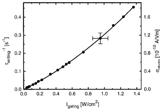
Fig. 4. Inverse time constant  $1/\tau_{\text{writing}}$  for hologram writing and photoconductivity  $\sigma_{\text{photo}}$  versus gating intensity at 488 nm. The curve is a fit according to  $\sigma_{\text{photo}} = aI_{\text{gating}} + bI_{\text{gating}}^2$ , where  $a$  and  $b$  represent fit parameters.
