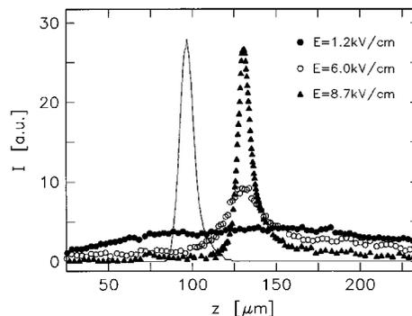
Fig. 3. Intensity profiles  $I(z)$  at the exit face of the waveguide measured for different externally applied electric fields  $E$ . The profiles are for the measurement shown in Fig. 2 and an input power  $P_{\text{in}} = 4.3$   $\mu\text{W}$ . For comparison, the solid curve shows the input beam profile (shifted for better viewing).
