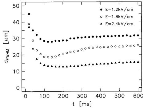
Fig. 4. Time evolution of the beam diameter  $d$  (FWHM) in the presence of different externally applied electric fields  $E$ . The input power of the He-Ne laser light is  $55 \mu\text{W}$ .
