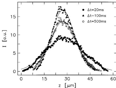
Fig. 5. Intensity profiles  $I(z)$  at the exit face of the waveguide measured for different time delays  $\Delta t$  after the He-Ne laser beam is switched on. The profiles are for the measurement shown in Fig. 4 and  $E = 1.8 \text{ kV/cm}$ .
