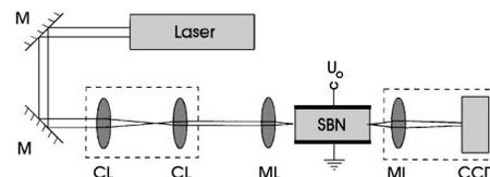
Fig. 1. Scheme of the experimental setup for spatial soliton formation in planar waveguides. M's, mirrors; CL's, cylindrical lenses; ML's, microscope lenses; U<sub>0</sub>, externally applied high voltage; SBN, SBN waveguide.
