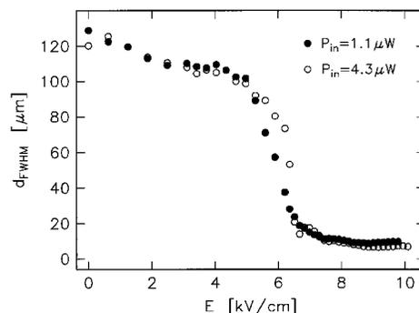
Fig. 2. Beam diameter  $d$  (FWHM) at the exit face of the waveguide as a function of the electric field  $E$  for two different input powers  $P_{\text{in}}$  of He-Ne laser light. The background illumination with green light ( $\lambda = 514.5$  nm) is  $\sim 30$  mW/cm<sup>2</sup>. All diameters are measured in the steady state.
