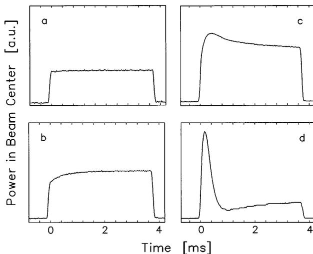
Fig. 4. Temporal evolution of the power in the center of the outcoupled light beam for several pulsed input powers (in milliwatts): a, 2.0; b, 3.9; c, 5.0; d, 14.1.
