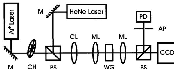
Fig. 1. Schematic of the experimental setup: M's mirrors; BS's, beam splitters; CH, mechanical chopper; CL, cylindrical lens; ML's, microscope lenses; WG, SBN waveguide; PD, photodetector; AP, aperture; CCD, CCD camera.
