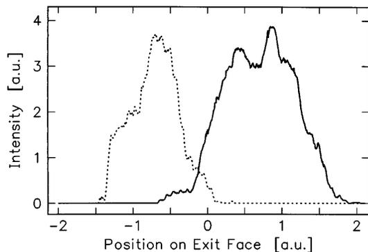
Fig. 5. Intensity distribution of the red probe beam on the exit face of the waveguide for high (10-mW, dashed curve) and low (1 mW, solid curve) cw input powers of the green pump beam. The red probe beam propagates under a small angle with respect to the green pump beam, intersecting it in the first half of the sample.
