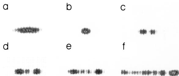
Fig. 3. Light intensity pattern coupled out of the end face of the waveguide for several cw input powers (in milliwatts): a, 0.1; b, 4.7; c, 12.0; d, 14.5; e, 15.5; f, 19.5.
