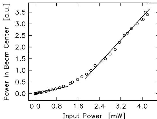
Fig. 2. Light power in the center of the outcoupled beam as a function of cw input power.
