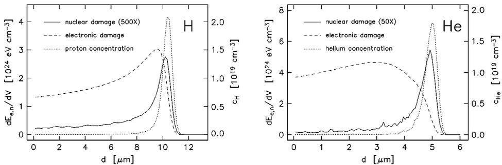
Fig. 1. TRIM simulation of implantation of 1 MeV  $\text{H}^+$  at a dose of  $2 \times 10^{15} \text{ cm}^{-2}$  (left), and 2 MeV  $\text{He}^+$  at a dose of  $1 \times 10^{15} \text{ cm}^{-2}$  (right). Nuclear and electronic energy losses,  $dE_n/dV$  and  $dE_e/dV$ , and H and He concentrations,  $c_{\text{H}}$  and  $c_{\text{He}}$ , are measured from the substrate surface
