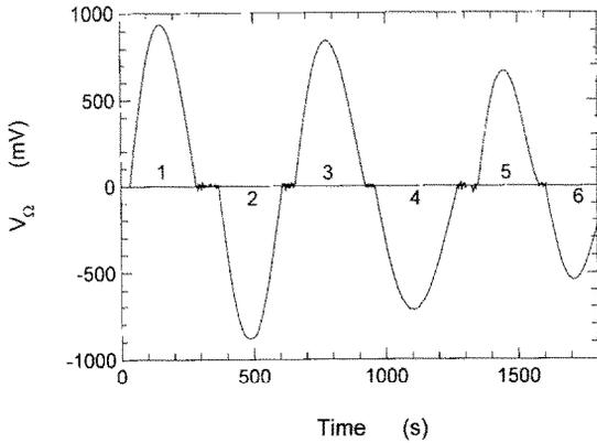
Fig. 2. Measured first harmonic evolution during self-stabilized holographic recording and erasure in LiNbO<sub>3</sub>:Fe (sample SC # 1, extraordinary polarization,  $I_1 = 5.1 \text{ mW/cm}^2$  and  $I_2 = 10.0 \text{ mW/cm}^2$ ). The odd cycles correspond to holographic recording, whereas the even cycles correspond to holographic erasure. Diffraction efficiency measured at the end of the cycles:  $\eta \approx 1$  and  $\eta \approx 0$ , respectively, for the odd and even cycles.
