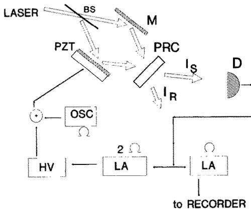
Fig. 1. Self-stabilized recording setup. M: mirror, PZT: piezoelectric supported mirror, BS: beamsplitter, PRC: LiNbO<sub>3</sub> crystal, D: detector, LA: lock-in amplifier, HV: high voltage amplifier for PZT, OSC: oscillator
